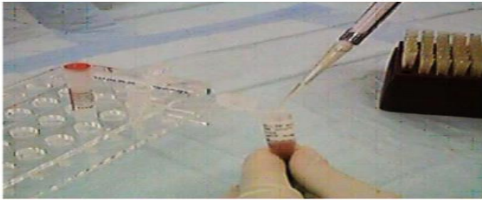
A. DNA polymerase and DNA sample are added to the tube containing PCR reaction buffer and dNTP.
